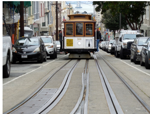
Car #10, headed up Jackson for Taylor Street, approaching the split. Note that the track takes a jog to accommodate the chafing bar and pulleys.
