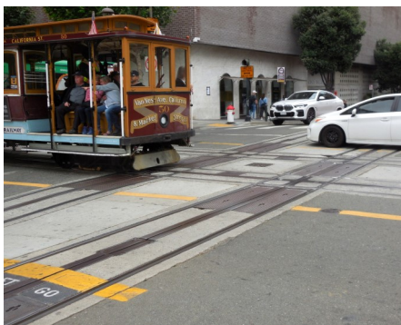
California Street car #50 rolls through the crossing. "LET GO" markings tell the Powell grip to release the cable.
