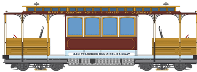
Above: Double-grip car (California Street) Below: Single-grip car (Powell-Hyde and Powell-Taylor)
