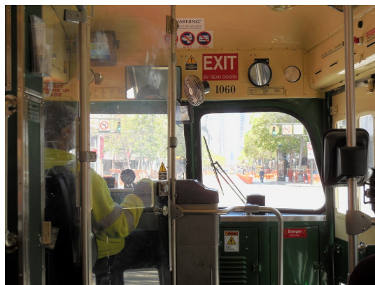
At the business end of the car: The fare box accepts bills only, and no change is given. The black box on the pole at right is the scanner for Clipper Cards, phone apps, etc.
