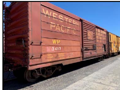
This was a Milwaukee Road 40' ribbed car that was sent to the Western Pacific after a Western Pacific Car was destroyed in a Milwaukee Road train accident. The Western Pacific put a nine foot door on the car and it became a Hotpoint appliance car. One of a kind. Very hard to model as models only have 8' and 10' doors.
