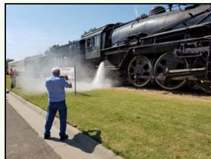
Blow down (former ATSF 3415)
