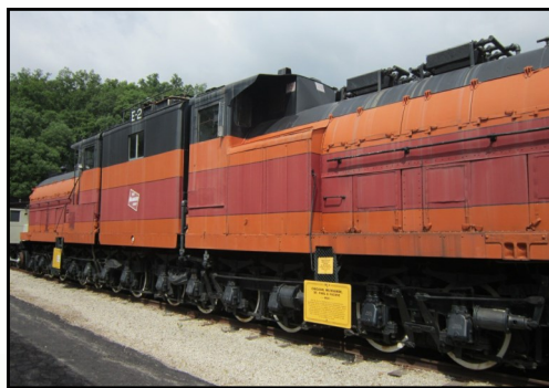
Milwaukee Bi-Polar Loco. The term bi-polar refers to the type of traction motors used. These had two poles that were part of the motor frame which reduced the size of the motor to allow it to fit within the power truck.
