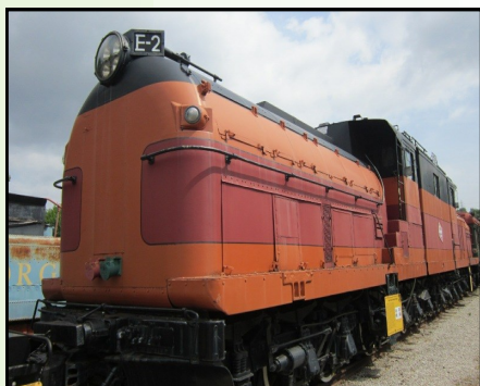
Milwaukee Bi-Polar Loco. The term bi-polar refers to the type of traction motors used. These had two poles that were part of the motor frame which reduced the size of the motor to allow it to fit within the power truck.
