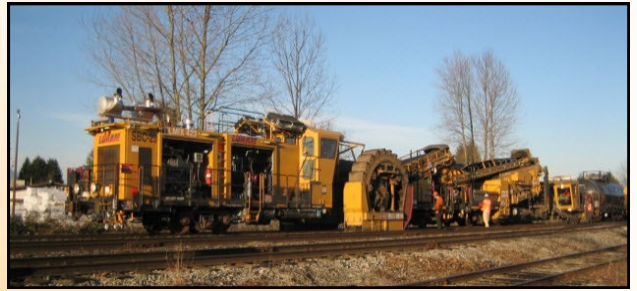
Track ballast cleaner in action. Loram MOW photo
